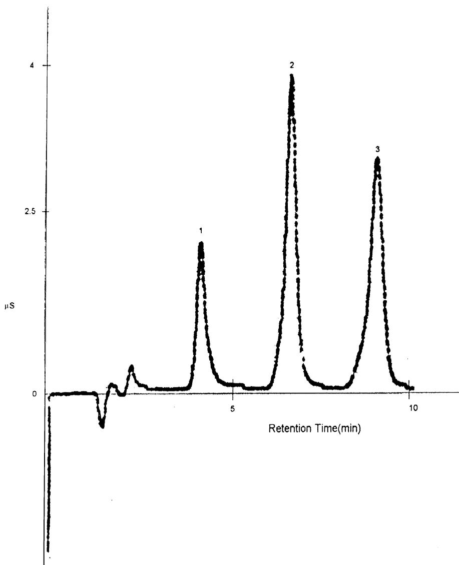
Fig. 3. Chromatogram of a sample containing L-cysteine and sodium pyrophosphate after oxidation to nitrate (1), phosphate (2) and sulphate (3).
